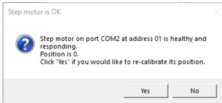
You will be asked if you would like to perform a re-calibration of retractor position. Click “Yes” and wait. After the calibration ends, take a test exposure of a bright target to ensure you see both rays. If your test image shows the problem was resolved, **Power Off** the retractor motor using remote power control.
