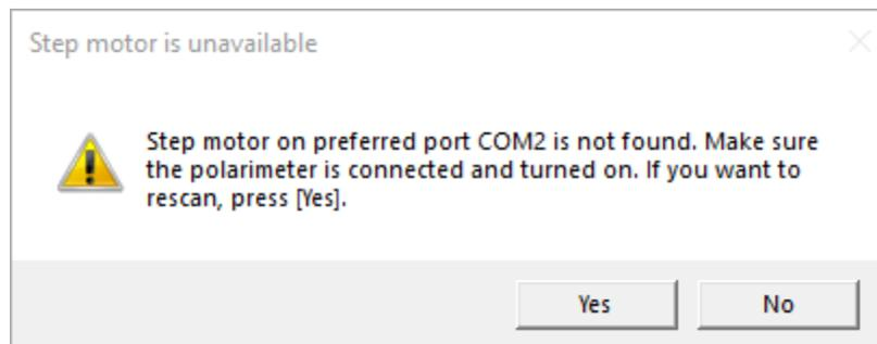
While powered off, click on the “Retractor” button, and observe a message box (do not close it). **Power On** the retractor motor and click “Yes” in the message box that was displayed to you by the Dipol-UF software. If everything is OK, the retractor motor will be identified, and you can continue observing in all regimes.
