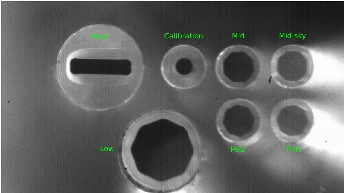
Figure 3: New FIES fiber exit slit plate illuminated from the side. The fibers are glued into a fused silica plate with precisely etched holes, and then polished. Clearly visible is the double cladding structure of the rectangular fiber (upper left). The dispersion direction is the y-direction.
