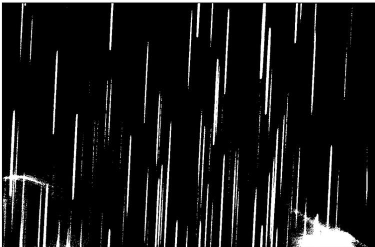
Figure 3.1: The comparison spectrum image taken with  $1152 \times 770$  pixels CCD in the first camera. The dispersion direction is on horizontal axis. The slit height is increased to the maximum. The non-aligned spectral lines are shown.
