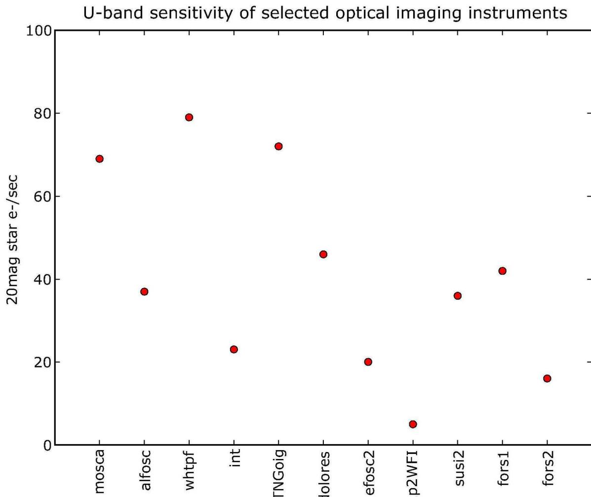
**Figure 2.** The *U*-band sensitivity of MOSCA and ALFOSC, compared to other instruments on La Palma and at ESO. The units of the plot are the same as in Figure 1.
