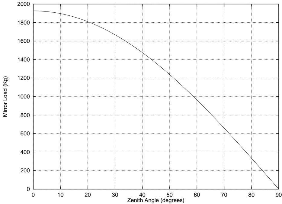
Figure 1: Mirror Load on Bellows verse Zenith Angle
