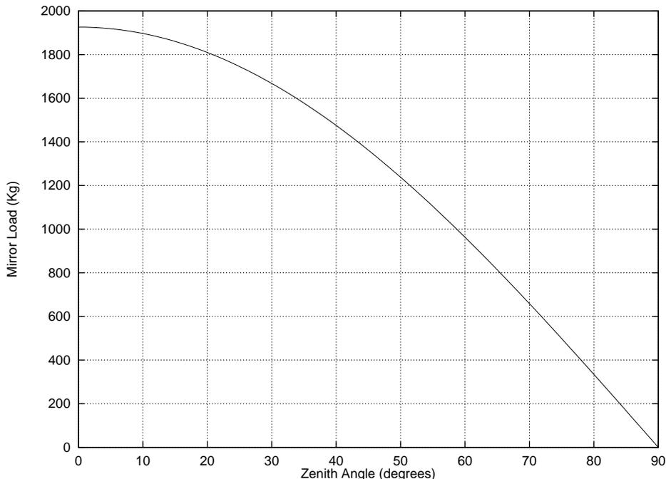
Figure 1: Mirror Load on Bellows verse Zenith Angle
