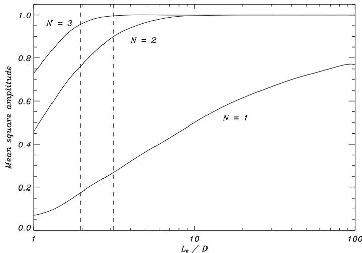
Figure 1: The mean square amplitude (the variance) of atmospheric aberration terms of radial order 1, 2 and 3 as function of the outer scale length  $L_0$  in units of telescope diameters, normalized to the amplitude at infinite  $L_0$ . The range of  $L_0 = 5\text{-}8\text{m}$  in the case of the NOT is indicated with vertical dashed lines.
