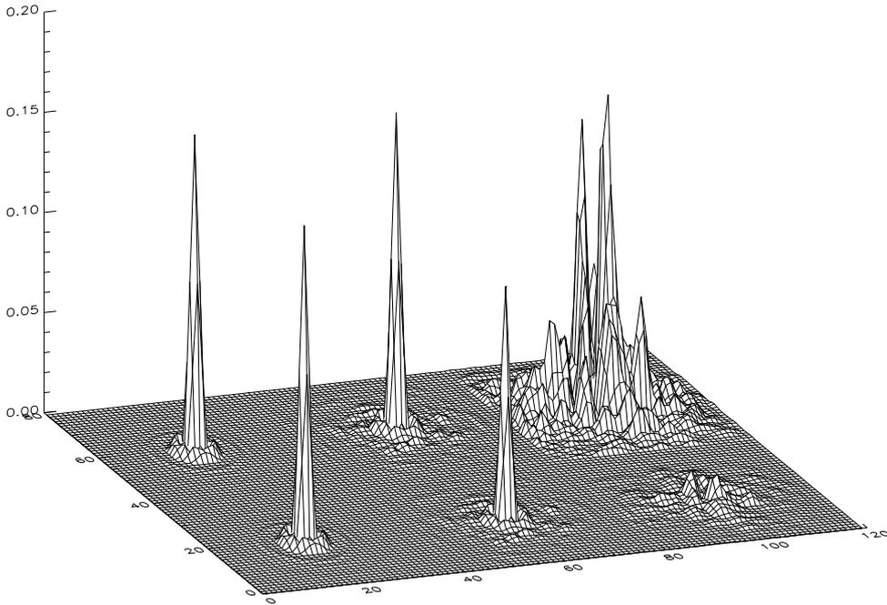
Figure 7: Point spread functions at a wavelength of 500nm, calculated from the phase-screens found from defocused images. Each PSF is shown in an array of  $0''.75$  size. *Front row, from left to right:* Un-aberrated PSF, PSF from map with 23 Zernike terms subtracted, PSF from complete map. Figures are normalized to the same total flux. *Back row:* Same PSF's, but normalized to same maximum local intensity.
