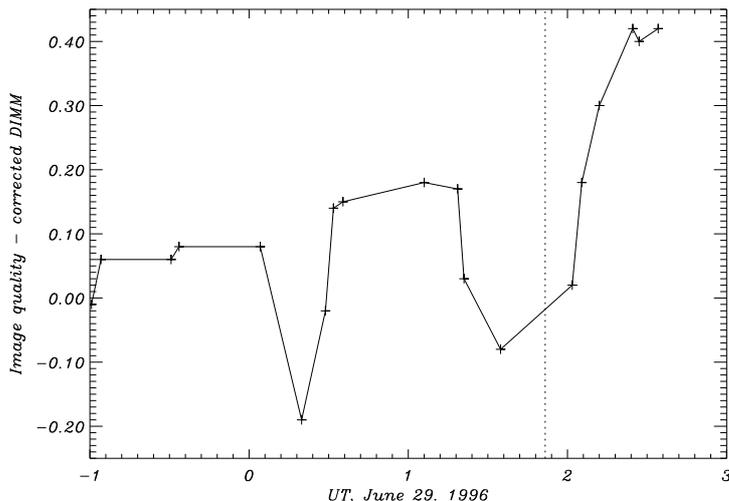
Figure 5: Difference between measured image quality and corrected DIMM measurement, as a function of time. The vertical dashed line indicate the moment when the telescope was turned from an up wind position to a down wind position.
