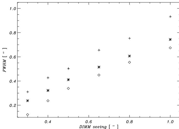
Figure 2: Correction of DIMM measurements in the case of an outer scale length of 8m. Shown is DIMM seeing (plus),  $L_0$  corrected DIMM seeing (asterisk) and tip/tilt corrected DIMM seeing (diamonds).
