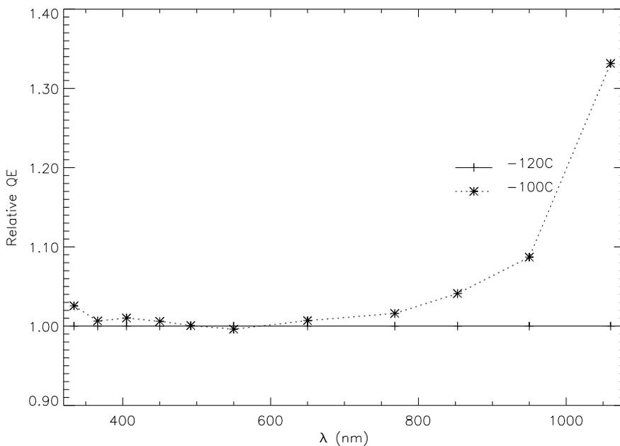
Figure 11: Quantum efficiency at  $-100^{\circ}\text{C}$  plotted relative to the QE at  $-120^{\circ}\text{C}$ . The improvement in QE from going to higher temperatures is quite large in the near-infrared.
