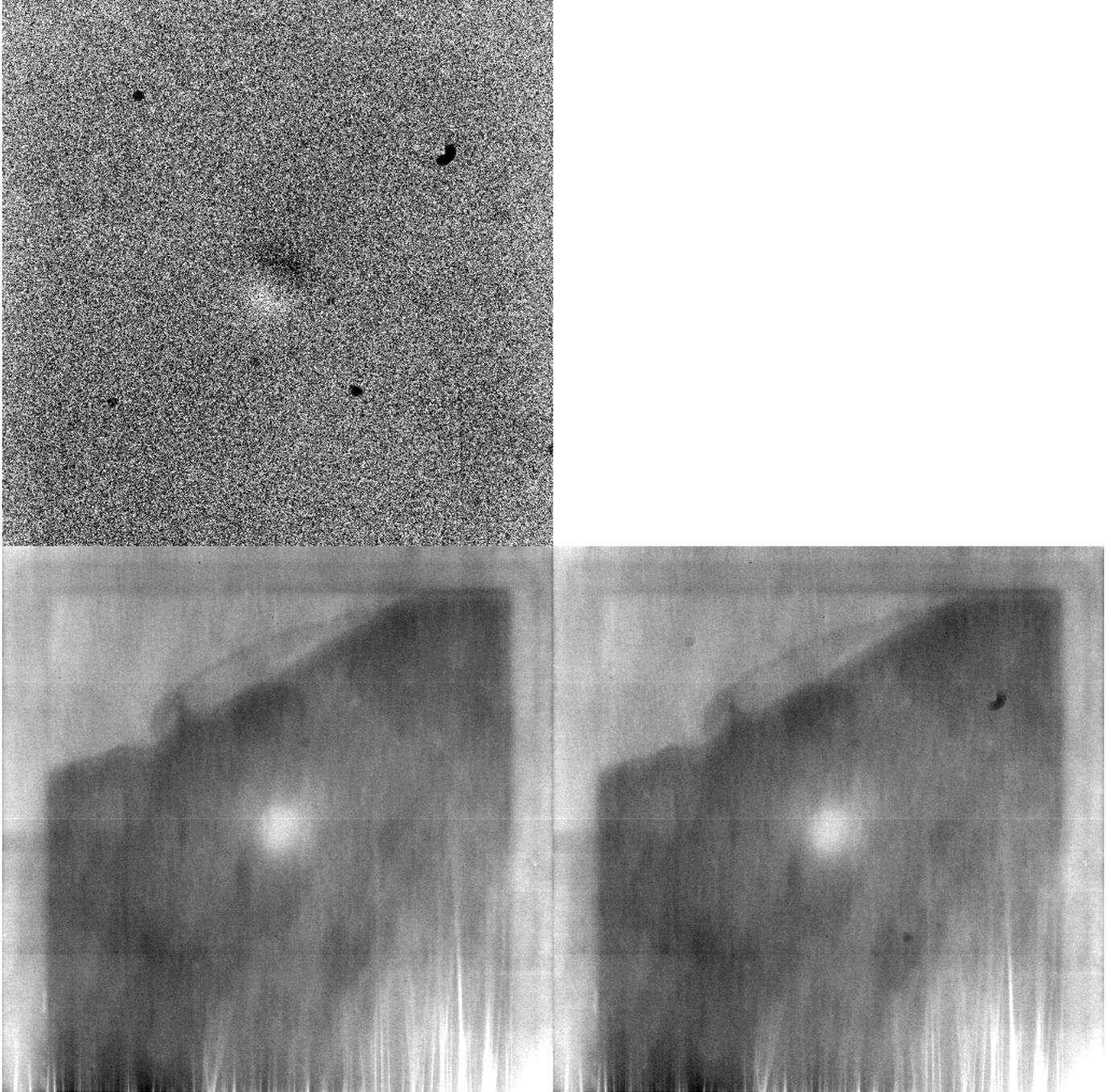
Figure 1: Flat field properties at 1060nm. *Lower left:* The greyscale cuts are set to  $\pm 8\%$  of the median level. *Lower right:* Five days later. *Top:* Ratio between the two flat fields, displayed with cuts of  $\pm 1\%$ . The local differences is due to new dust specks arriving and a changed distribution of scattered light.
