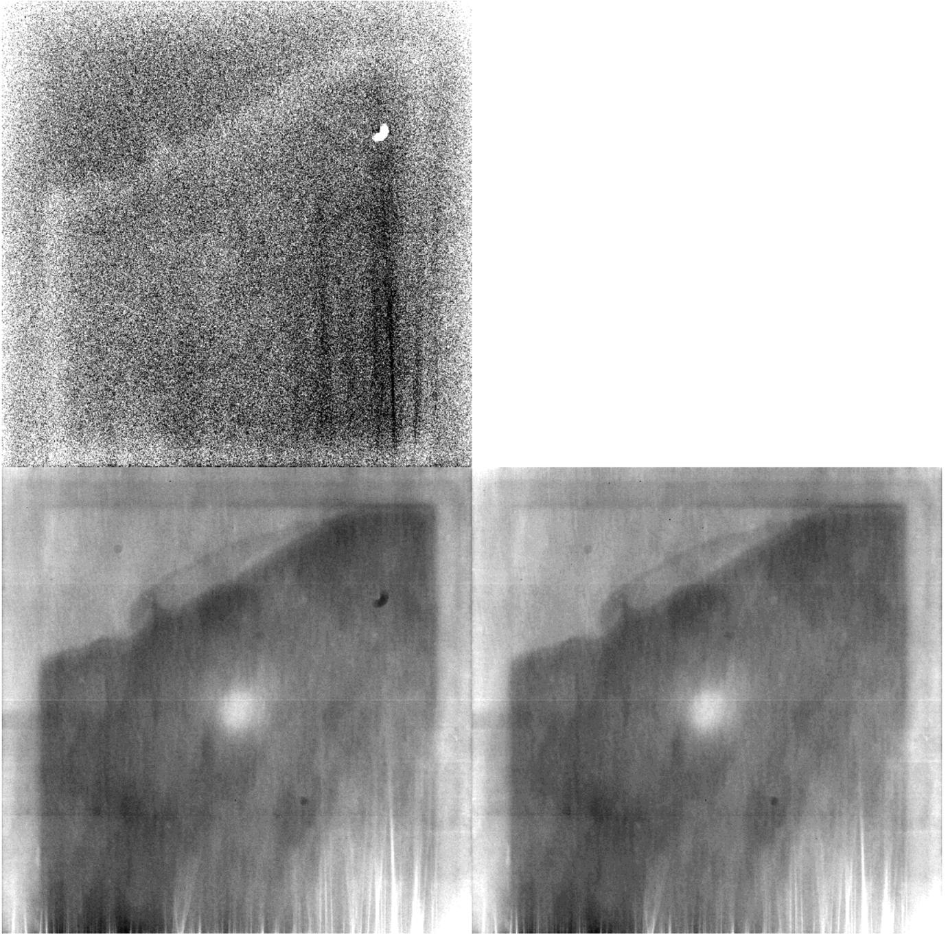
Figure 12: Flat field dependency on temperature at 1060nm. *Lower left:* CCD at  $-120^{\circ}\text{C}$ . The greyscale cuts are set to  $\pm 8\%$  of the median level. *Lower right:* CCD at  $-100^{\circ}\text{C}$ . *Top:* Ratio between the two flat fields, displayed with cuts of  $\pm 1\%$ . In the lighter areas, the QE has increased at  $-100^{\circ}\text{C}$  relatively to  $-120^{\circ}\text{C}$ . Also, a dust speck has moved and the reflections off the bonding wires have changed.
