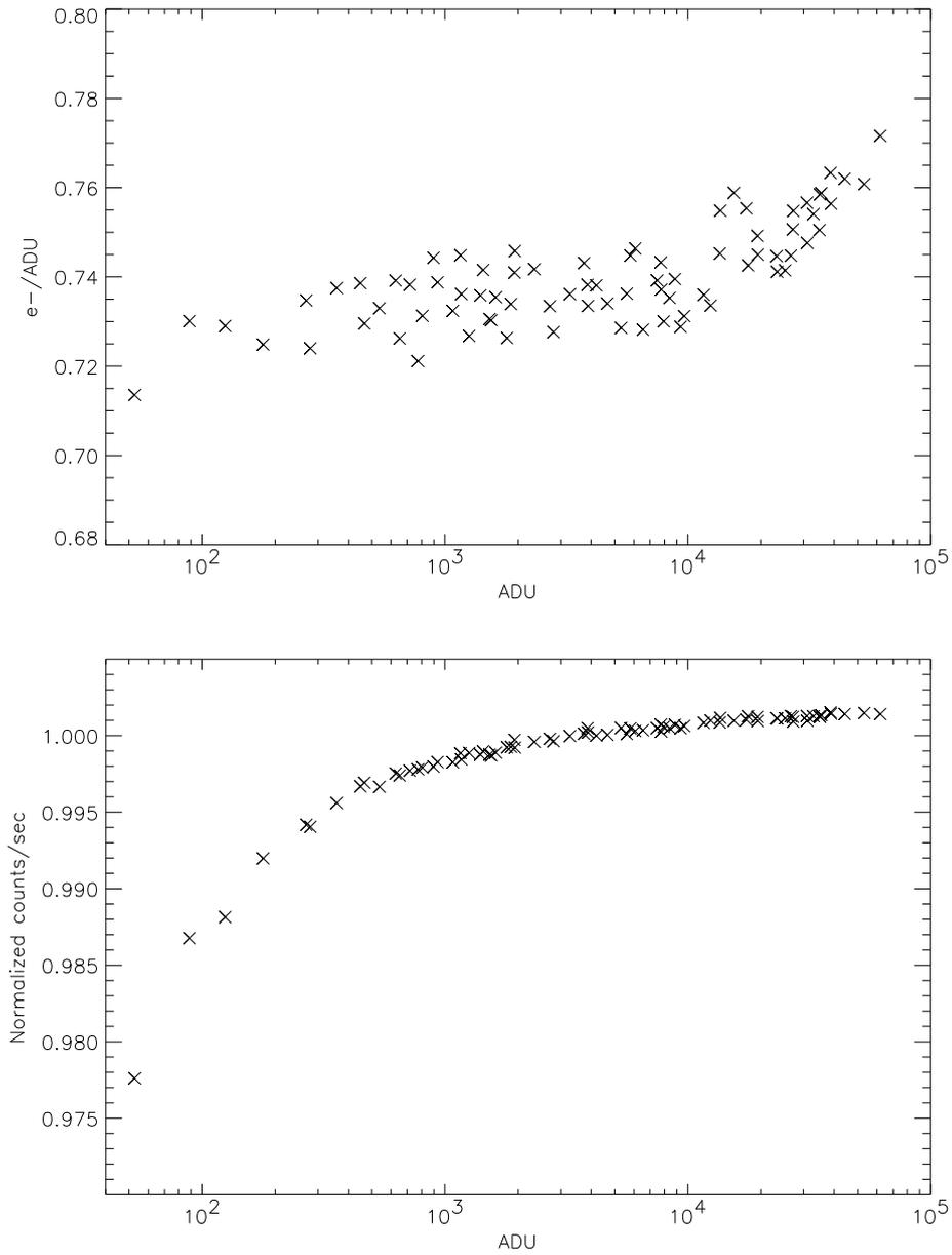
Figure 5: Linearity data for amplifier A in high gain mode. *Top*: Gain versus exposure level measured from noise statistics. *Bottom*: A plot of ADU per second versus total exposure time, corrected for shutter delay.
