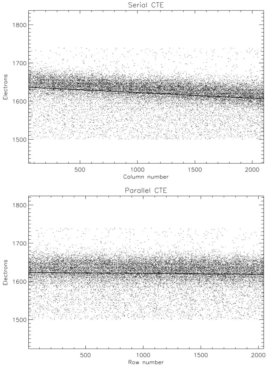
Figure 9: Plot of  $^{55}\text{Fe}$  K- $\alpha$  peak counts versus row and column position, used for measuring CTE. The gradient along the rows shows a slight loss during serial transfers, while parallel shifts are near perfect.
