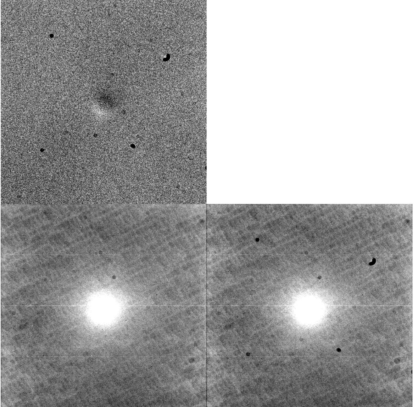
Figure 2: Flat field properties at 550nm. *Lower left:* The greyscale cuts are set to  $\pm 2\%$  of the median level. *Lower right:* 5 days later. *Top:* Ratio between the two flat fields, displayed with cuts of  $\pm 1\%$ .
