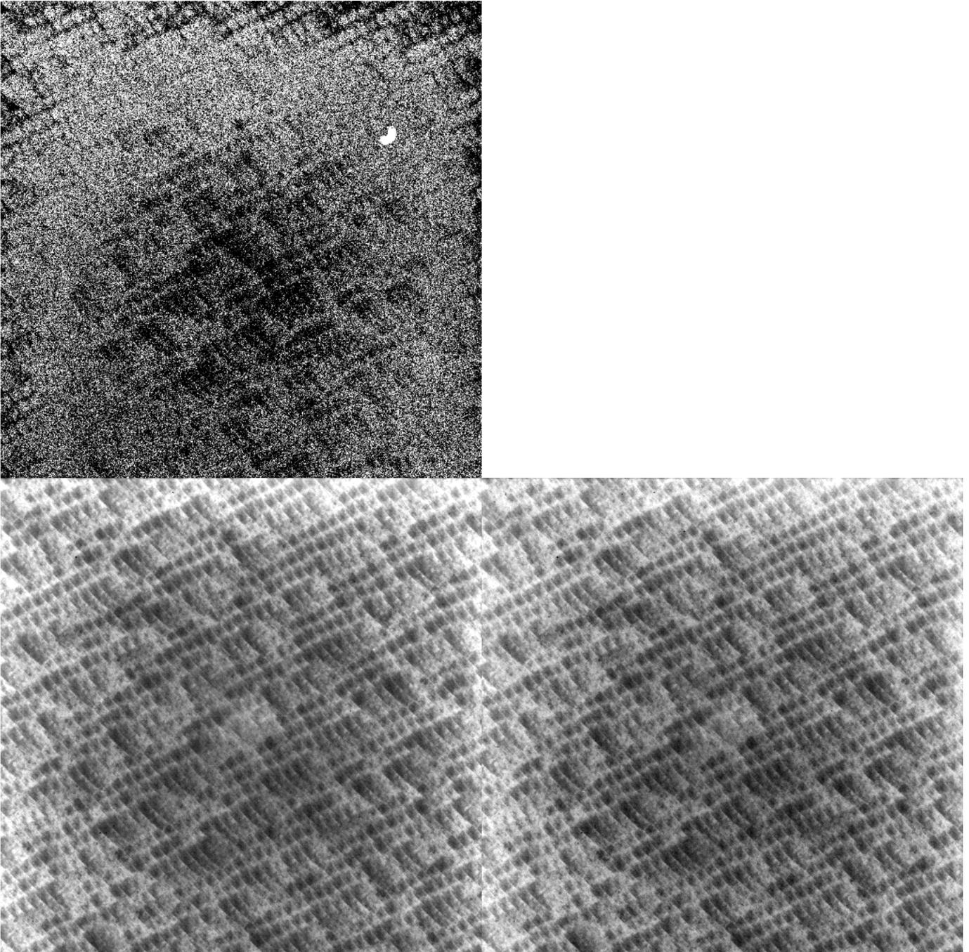
Figure 13: Flat field dependency on temperature at 334nm. *Lower left:* CCD at  $-120^{\circ}\text{C}$ . The greyscale cuts are set to  $\pm 15\%$  of the median level. *Lower right:* CCD at  $-100^{\circ}\text{C}$ . *Upper left:* Ratio between the two flat fields, displayed with cuts of  $\pm 1\%$ . In the lighter areas, the QE has increased at  $-100^{\circ}\text{C}$  relatively to  $-120^{\circ}\text{C}$ .
