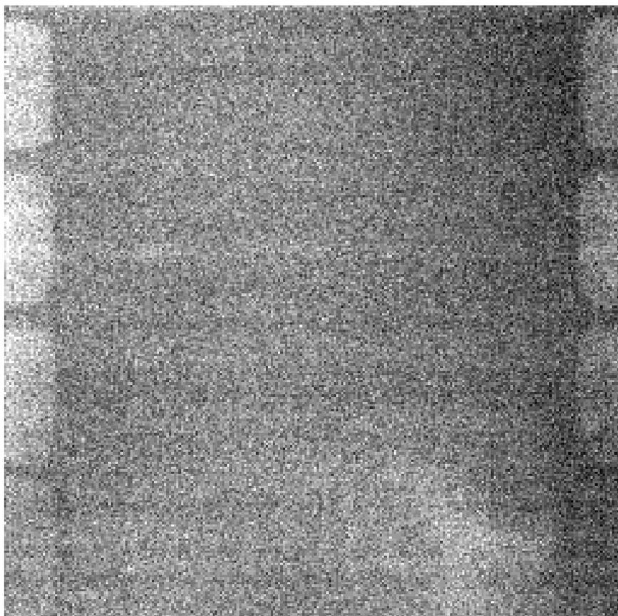
Figure 18: Dark current and residual image distribution for an 1 hour measurement using 4 by 4 pixel binnig. The average level is  $8.8e^-/\text{pixel}/\text{hour}$ , but some variation can be seen. At both sides, bands with increased flux appear, along with a triangular structure in the lower right corner. There are no hot pixels or columns to be found.
