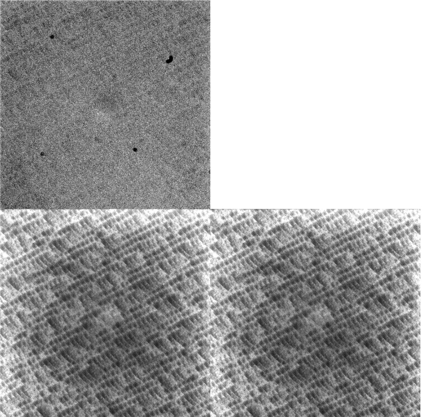
Figure 3: Flat field properties at 334nm. *Lower left:* The greyscale cuts are set to  $\pm 15\%$  of the median level. *Lower right:* 5 days later. *Upper left:* Ratio between the two flat fields, displayed with cuts of  $\pm 2\%$ .
