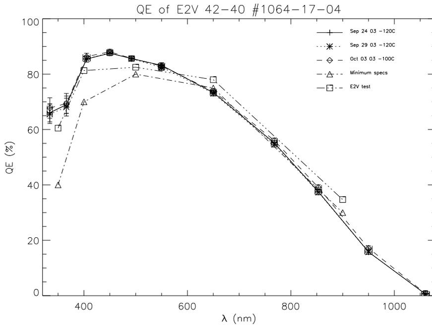
Figure 10: Quantum efficiency versus wavelength for the CCD42-40 at  $-120^{\circ}\text{C}$ , measured twice at  $-120^{\circ}\text{C}$  and, slightly above, at  $-100^{\circ}\text{C}$ . These are drawn with horizontal bars marking filter FWHM and vertical bars showing the Pixel Response Non-Uniformity. Also shown are E2V minimum specifications (triangles) and test data (squares) at  $-30^{\circ}\text{C}$ .
