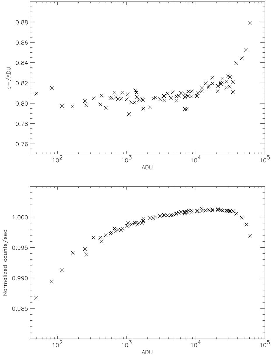
Figure 6: *Top*: Gain versus exposure level measured from noise statistics for amplifier B in high-gain mode. *Bottom*: A plot of ADU per second versus total exposure time, corrected for shutter delay. Data is again for amplifier B in high-gain mode.
