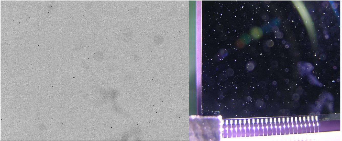
**Illustration 7: Left: An approx. 900x700 section of a 550nm flatfield. Right: The corresponding area photographed with oblique illumination.**
