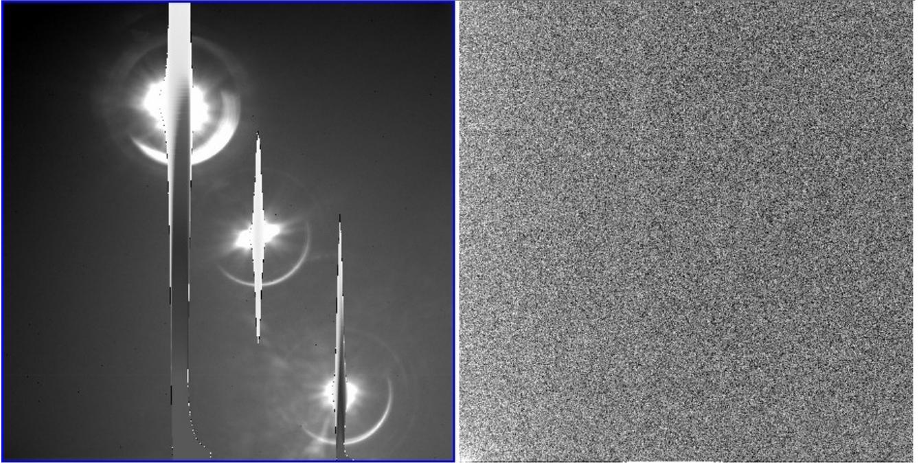
Illustration 8: Left: Saturated exposure. Right: First 100sec dark out of 10.
