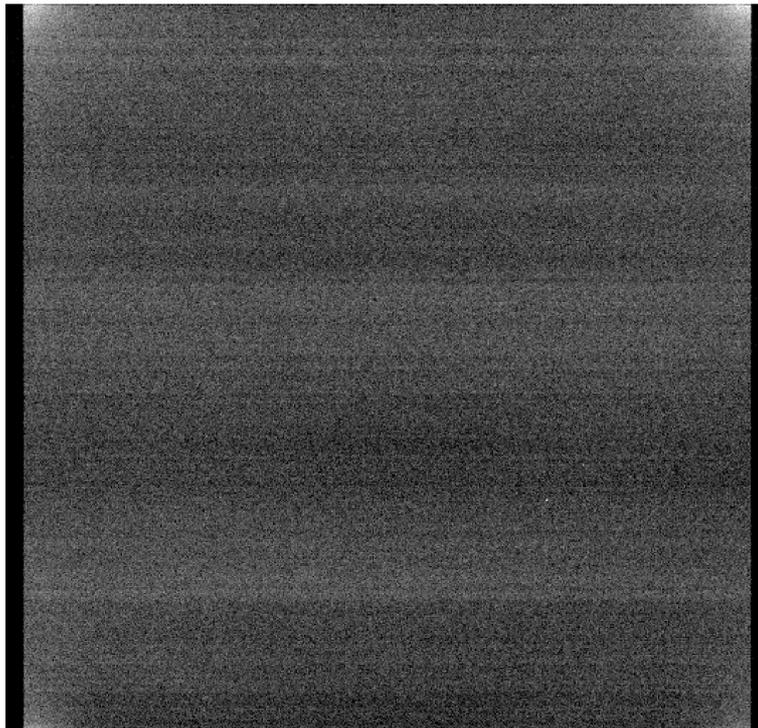
**Illustration 10: Map of 20 stacked dark integrations, for a total integration time of 10 hours. The image area is clearly brighter than the overscan region, and brightest near the corners. Horizontal bands appear due to bias level fluctuations.**
