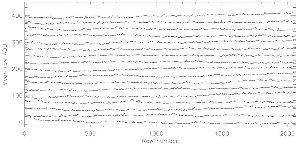
**Illustration 11: Vertical profiles of 17 full-frame biases. A separation of 25 ADU between profiles has been added.**
