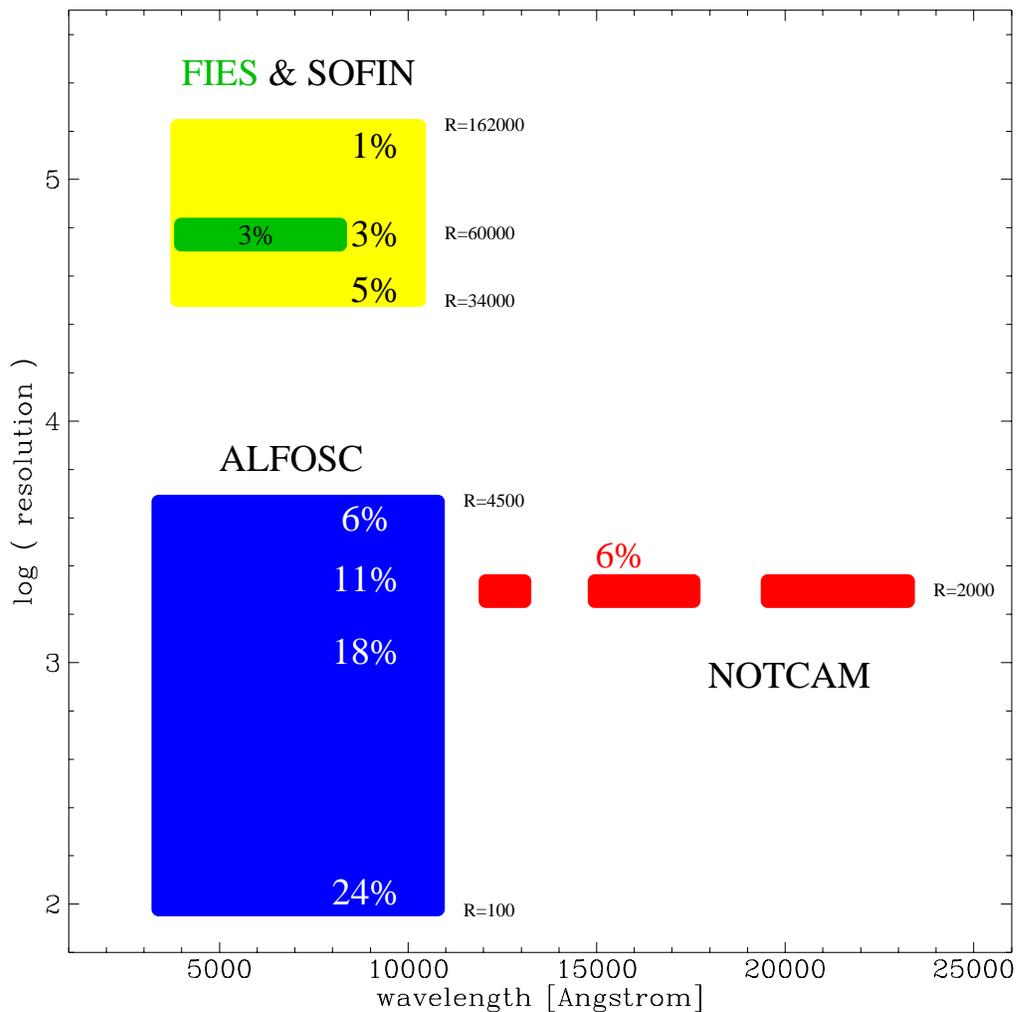
Figure 4: Current spectroscopic functionality and peak efficiency in a plot of spectral resolution versus wavelength. Note that SOFIN is depicted as yellow; FIES as green.
