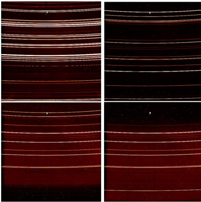
Figure 5: NOTcam Argon spectra taken with recently purchased calibration lamps. The high cuts are at 4000 ADU and the exposure times were 10 seconds. Top: J and H band. Bottom: K' and K band
