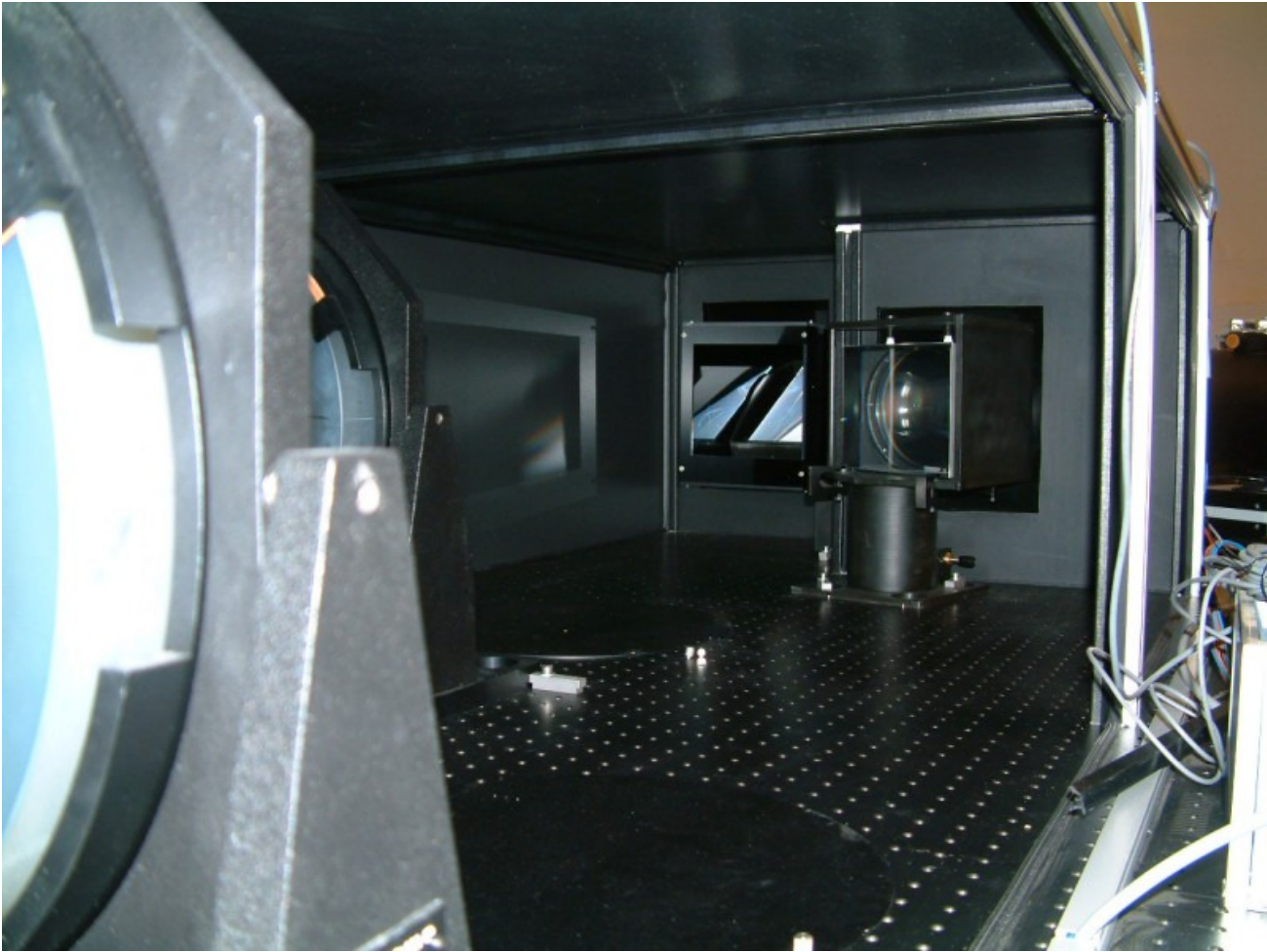
Fig. 1 View into the spectrograph when opened; on the left the two off-axis collimators seen from behind; on the right the shiny grating, and even further right the cross disperser. The exposure meter was not yet installed at the time this picture was taken.
