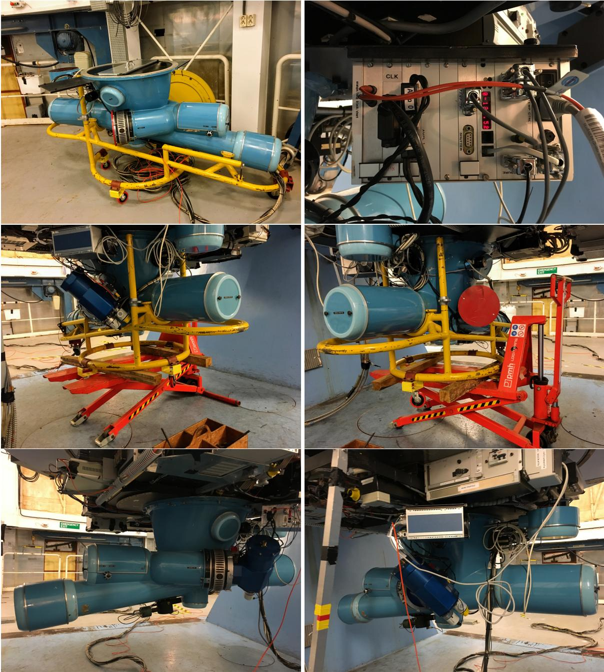
Figure 4: Shown spectrograph in the storage position with the cover removed and the Loral CCD controller with permanently connected electronics cables (top row). Location of the fork lift when mounted on the telescope with the rotator at rot-pos 0 (middle row). SOFIN mounted with rot-pos -90 (lower row). The location of the cross-dispersion prism flipping knob is seen.
