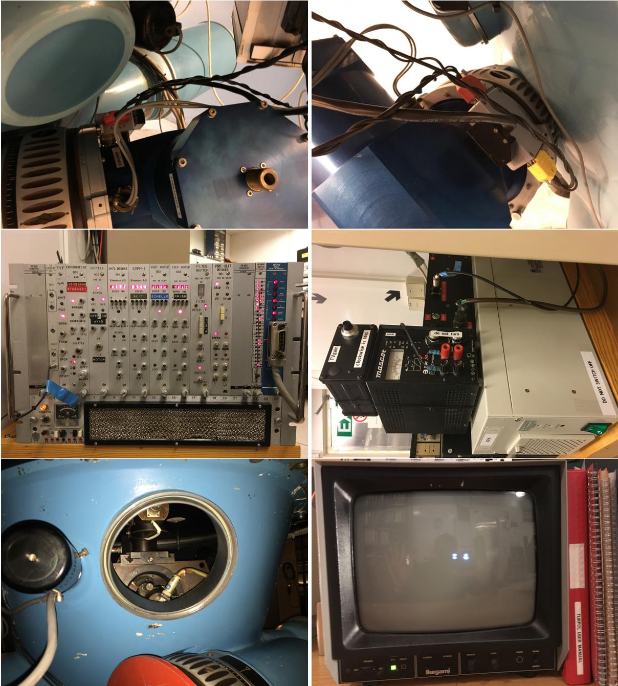
Figure 5: The five connecting cables to the CCD dewar (top row). The CAMAC crate and the two power supplies atop of the control computer (middle row). The slit decker location with the slit hatch removed and the two polarized beams from a star as seen on the slit viewing camera (bottom row).
