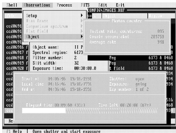
Figure 5.2: The snapshot of the control program screen after the object exposure has started shows the exposure watch window and the photon counter window.
