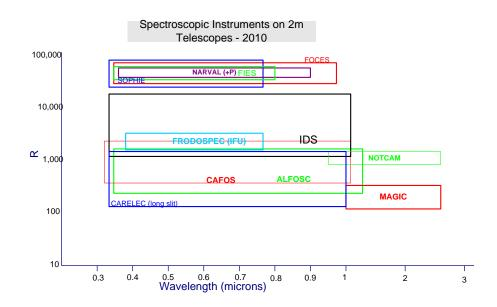
Spectroscopic Instruments on 2m Telescopes – 2012+ optimal suite
