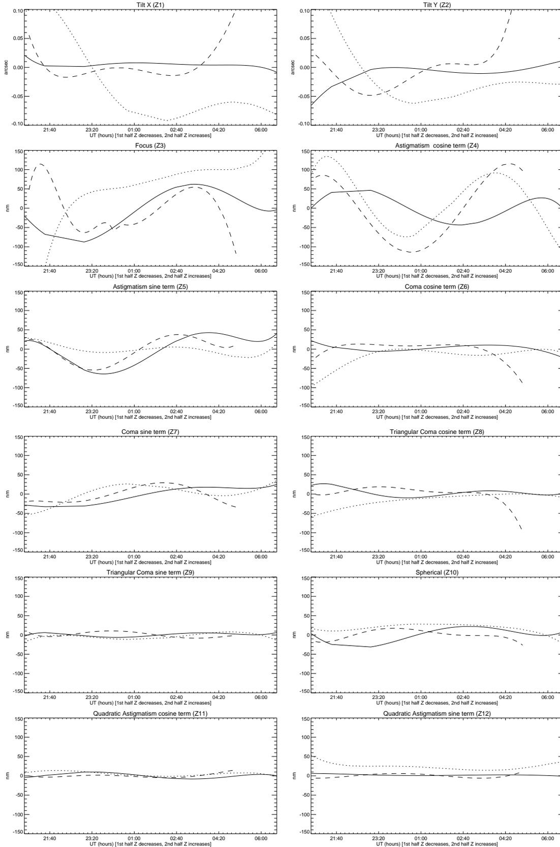
Figure 1: Zernike evolution against time for 28/3/02 (solid), 11/2/03 (dots) and 11/4/03 (dashes).
