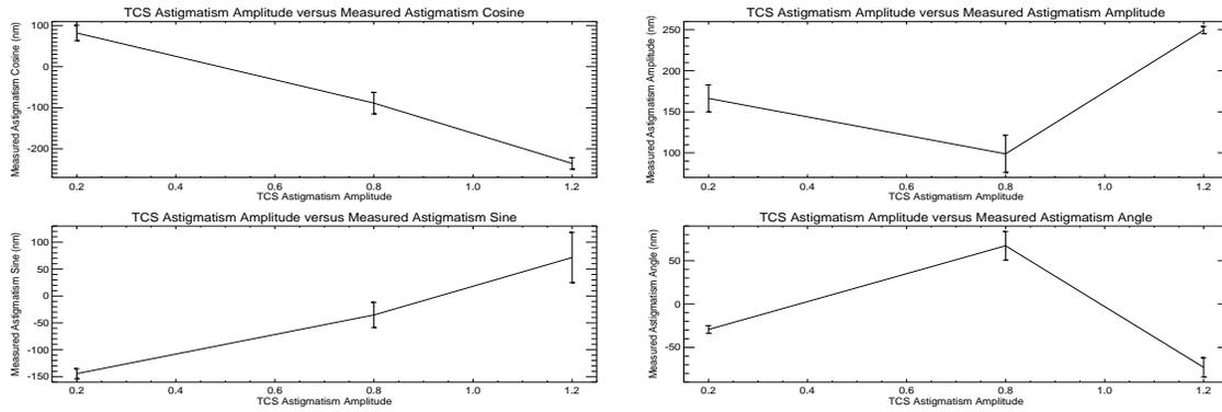
Figure 10: Relationship between applied TCS astigmatism amplitude versus measured Zernikes Z4 and Z5, Cosine and Sine respectively.
