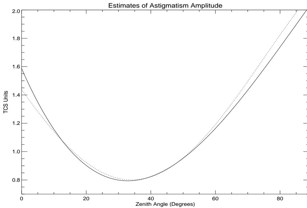
Figure 8: Two estimates of the Astigmatism Amplitude versus Zenith Angle. The solid line is a polynomial fit and the dotted a best guess Cosine fit.
