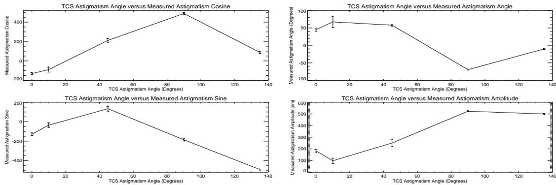
Figure 12: Relationship between applied TCS astigmatism angle versus measured Zernikes Z4 and Z5, Cosine and Sine respectively.
