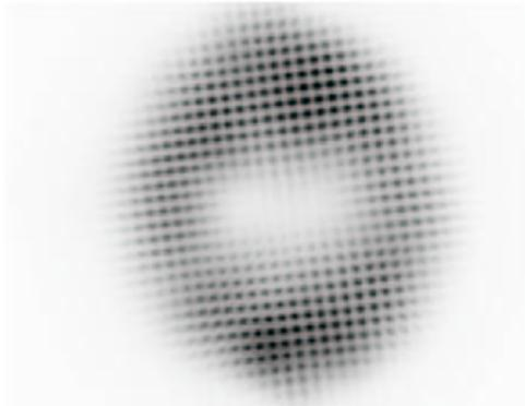
Figure 1: This is a typical WFS mask stellar image taken on night of 25 March 2004. Note the vertical elongation of the image with a perpendicular elongation of the centre obscuration.
