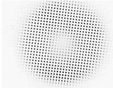
Figure 2: Typical WFS calibration mask image.
