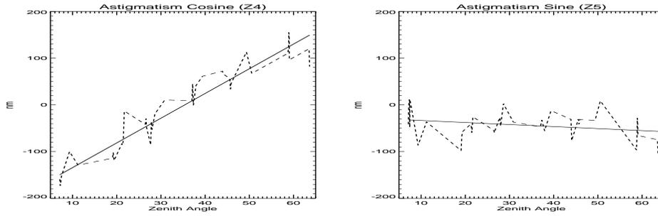
Figure 9: Zernike terms (Z4 and Z5) of the astigmatism with straight line fits.
